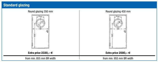
\* Standard glazing profiles made of steel with transparent fire resistant glazing. Glass for indoor use only, UV resistant as per EN ISO 12543-4 Section 6, also suitable for areas exposed to sunlight (shield glass from direct halogen light radiation. Glass can only be used within a temperature range of -20 to +50°C).
