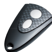
Micro-Novotron 512 Design 2-Kanal, 433 MHz, KeeLoq-Wechselcode
