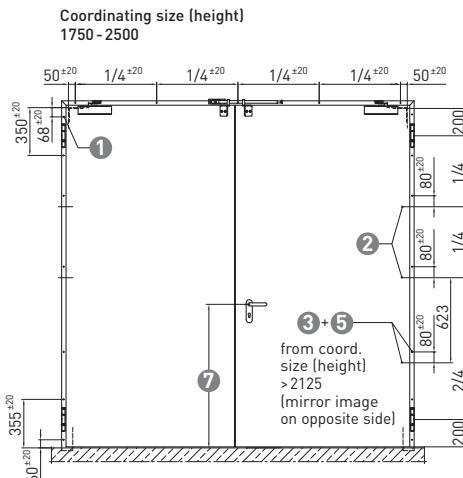
**Sealing of smoke protection doors (version S<sub>200</sub>):**
