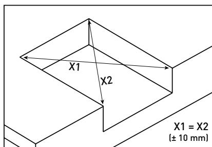
Instruction: The leveller must be installed so that it is perfectly horizontal across its width. If not, leveller operation may be adversely affected. There is also a risk of damage to the leveller.
